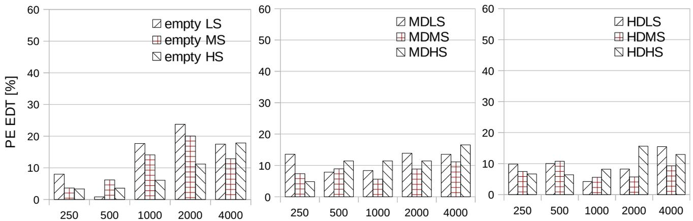
**Figure 5:** Early decay Time (EDT) Prediction Errors [%]
